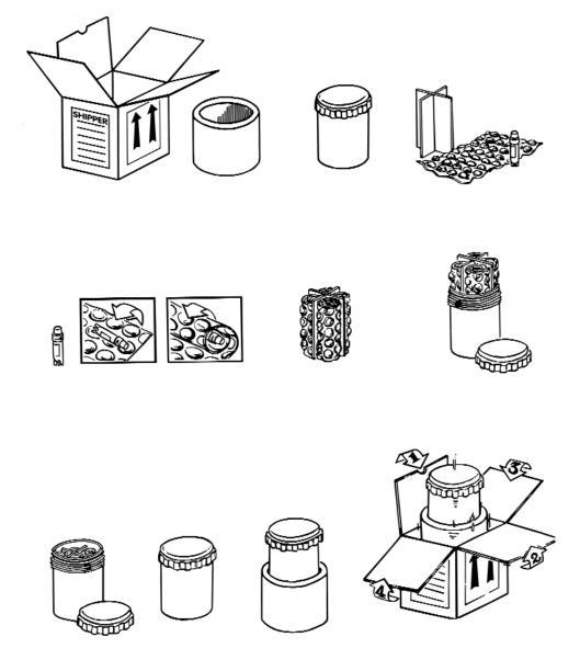
*Note 1:* This diagram shows just one example of an acceptable packaging system. Several primary containers (cryovials) may be enclosed in a single secondary container, if the total volume of all the primary containers does not exceed 50 ml and there is no contact between them.
