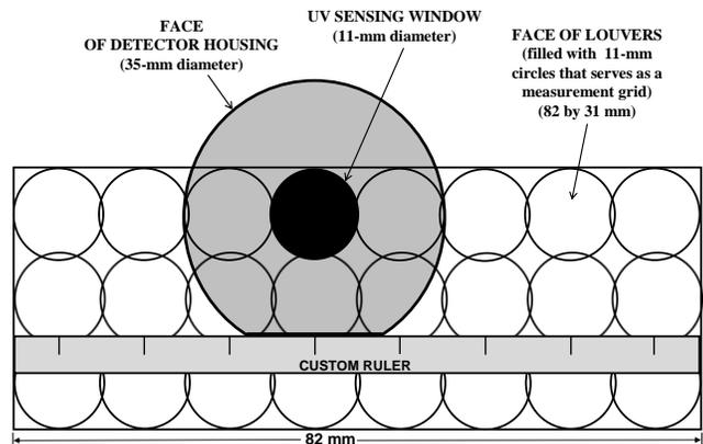
The measurement procedure, which can be used for the louvered face of almost any commercially available upper-room UVGI fixture, was designed so positioning the UV detector and measurement of irradiance for a specific location on the louvered face is precise, relatively simple, and rapid. For illustrative purposes, the hypothetical louvered face shown in Figure 6 is used as a basis for explaining the measurement procedure described below:
