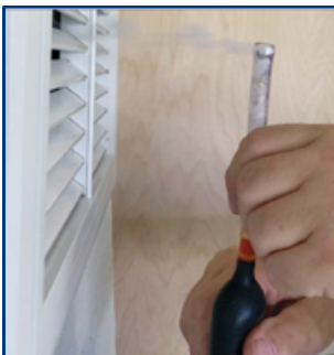
Figure 23. Smoke generated tube in order to visualize the movement of air.
