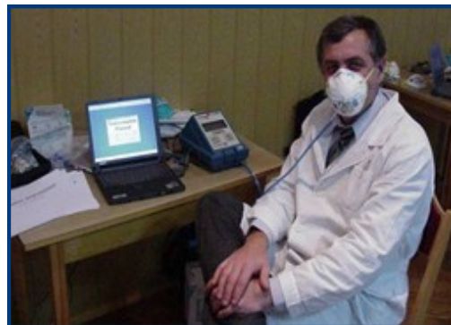
Figure 26. Health worker just completed and passed a quantitative fit test to ensure proper fit.
