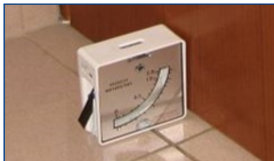
Figure 24. Swinging vane anemometer used to visualize air moving underneath a door.
