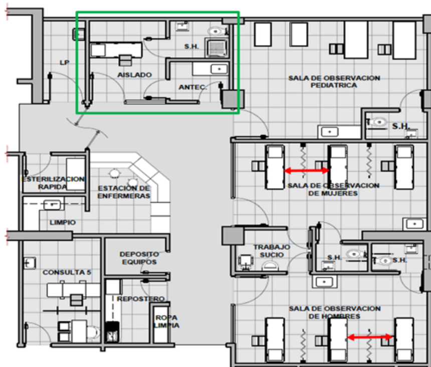
Figure 16. Inpatient Infectious Disease Ward (airborne precautions). The rooms are separated by life stages and by sex, beds must be separated by at least 1.5 m. It also has a respiratory isolation room with a private bathroom (in green).
