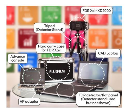
Figure 12. Labelled Fujifilm FDR Xair core system. Image courtesy of DOPASI.
