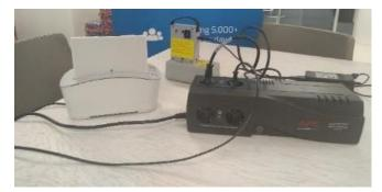
Battery chargers for Delft Light generator and detector
