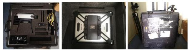
Figure 11. The packaging of (a) the generator and accessories, (b) the detector, and (c) the carrying case (external). *Images courtesy of CIDRZ.*
